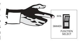
e. If you are not ready to cook, place the FUNCTION SWITCH in the SIMMER position. This will cause the heating element to shut off and the internal thermostat to maintain the water temperature at around 205°F.
